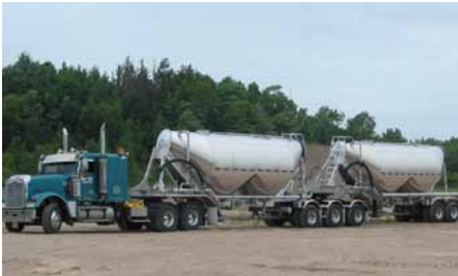
B-trains like this one use less fuel per tonnage hauled.
